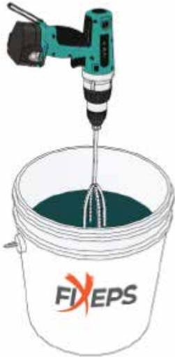
The EPSBLOCK mortar (FIXEPS) to be used must be prepared in small batches. 25 kg FIXEPS mortar is sprinkled on 6 liters of clean water. The prepared mortar is allowed to mature for 5 minutes and then mixed again.
